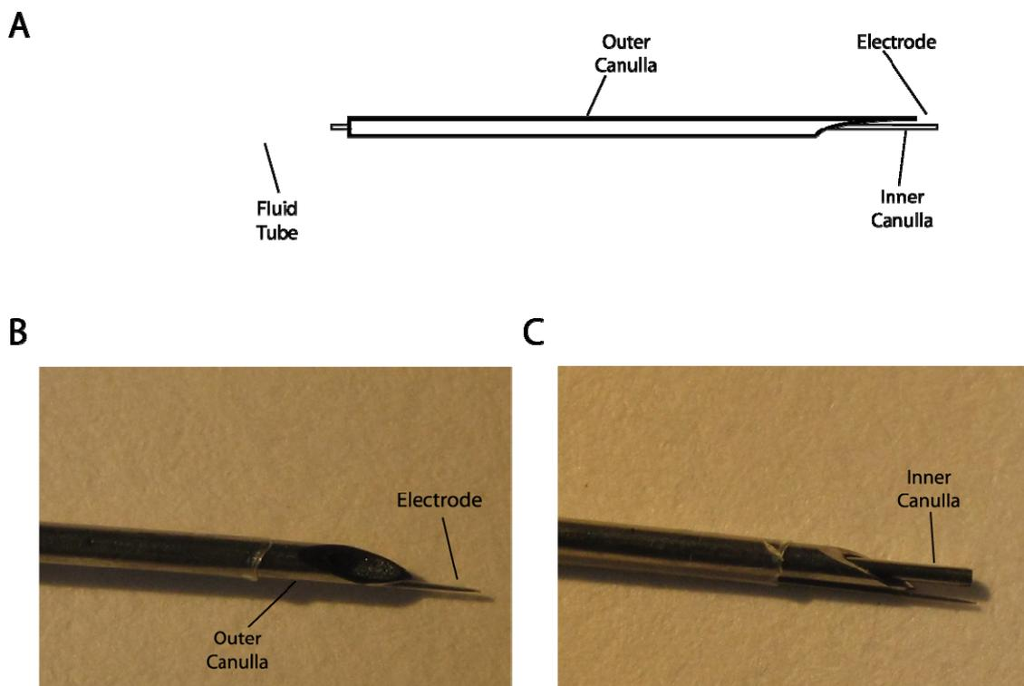
**Figure 1** The inactivation Cannula system. **A** A cartoon description of the Cannula. See text for details **B**. The electrode attached to the outer Cannula attached by a shrink tube. Notice that the electrode is attached to the longer side of the Cannula. **C** The inner Cannula inside the outer Cannula.
